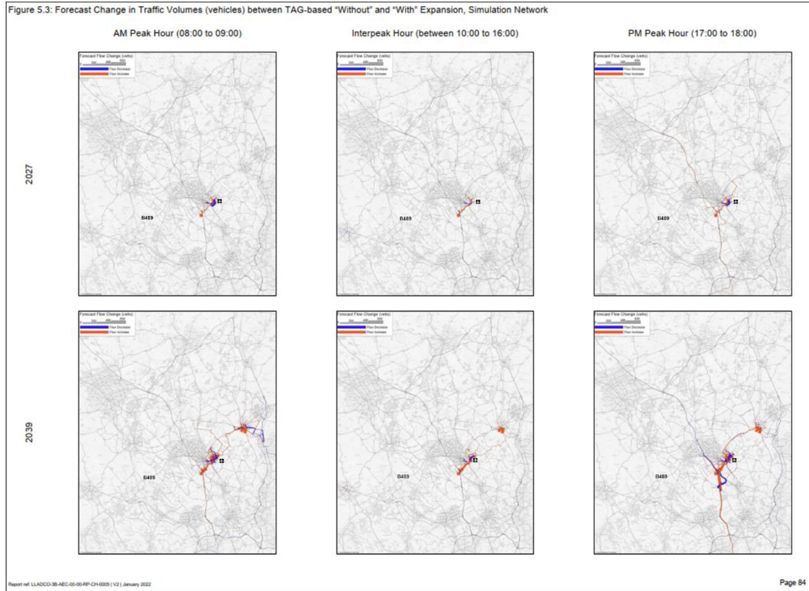
Figure 16 (Part 1 / 2) – Forecast Change in Traffic Volumes (vehicles) between TAG-based “Without” and “With” Expansion, Simulation Network
